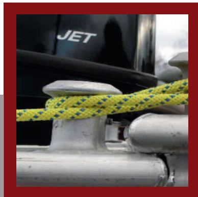
Exclusive ONELink System Allows multiple R ONE Series® boats to interconnect. ONELink creates a quick rigid connection in multiple configurations and disconnects in seconds.
